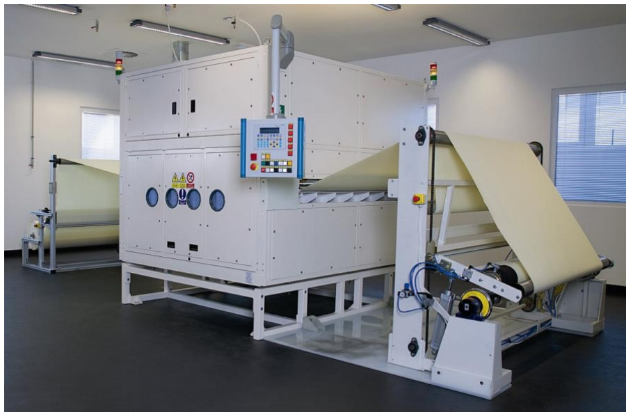
Figure 6. Nozzle-less production electrospinning line (Nanospider™)
